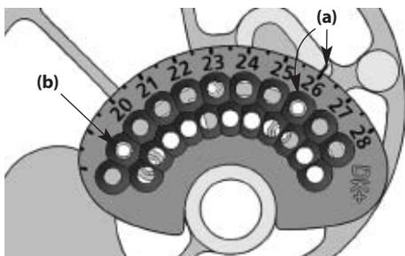
**Example:** the mod is positioned for a 26" draw length.
