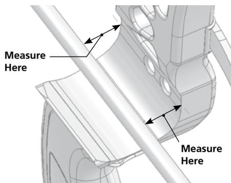
**Figure 3: Determining Center Shot** your bow (see **Figure 3**). This is a good starting point when tuning your Diamond bow. Keep in mind, not all bows tune at exact center shot due to the variances in arrow spine, hand position, and your specific bow poundage. Adjust your arrow rest until the two measurements are equal.
