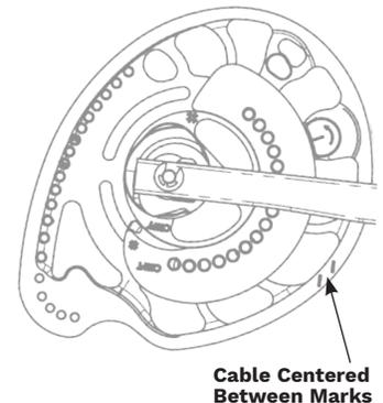
**Figure 5: Cam Timing**
