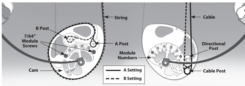
Figure 2. The Nuclear Ice bottom cam, (both sides).
